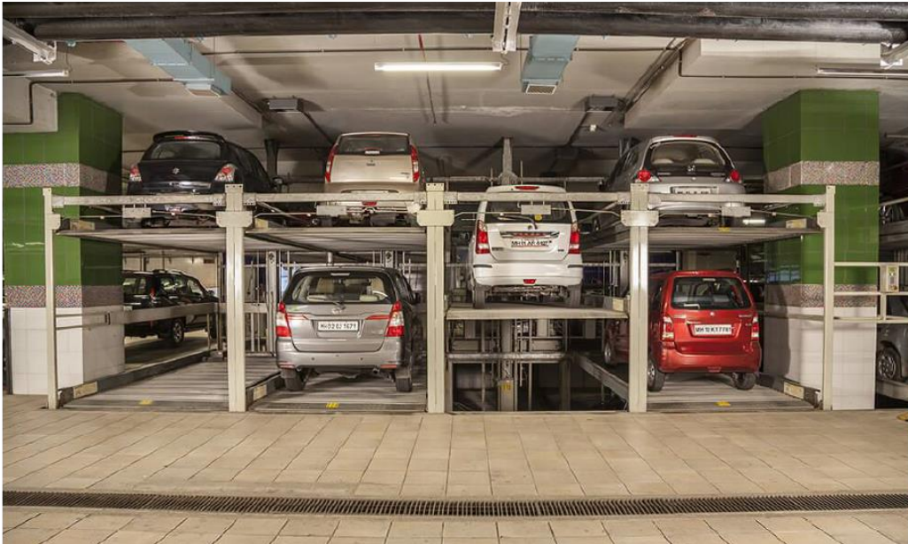
Figure 6.19: Multi-level car parking (example)
